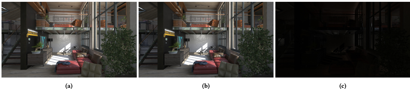
Figure 1: (a) The reference path traced image of loft scene. (b) Rendered with the proposed method. (c) Difference between (a) and (b) shows the error from the method. Rendering time and ray casting time were reduced by 6 % and 12 %, respectively, using our method.
